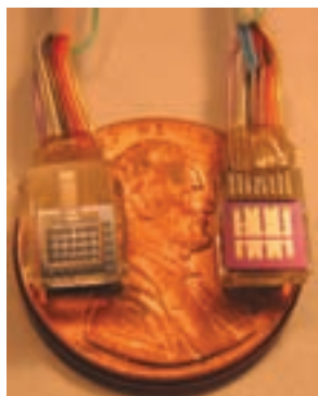
◀ Figure 1: Picture of the MEMS device showing the Pyrex macroreservoir (left) bonded to the silicon chip (right). The metallic layer on the silicon chip controls the opening of micro-wells allowing vasopressin out of the macroreservoir.
